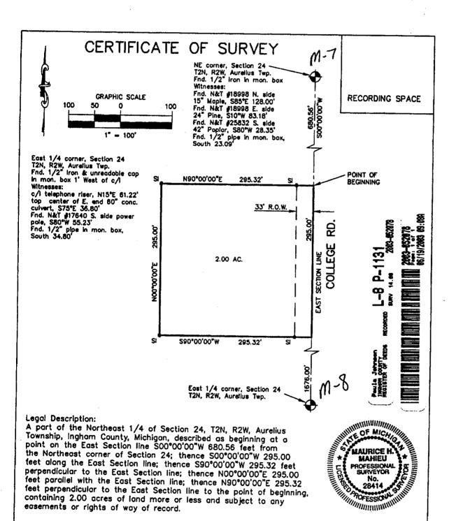
The basis of bearing for this survey is based on assuming  $$00^{\circ}00'00''W$$  on the East Section Line.
