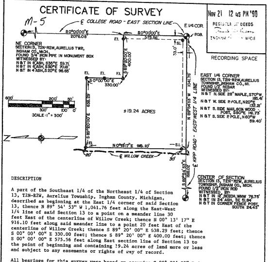
All bearings for this survey were based on assuming S 00° 00' 00" E for the East section line.
