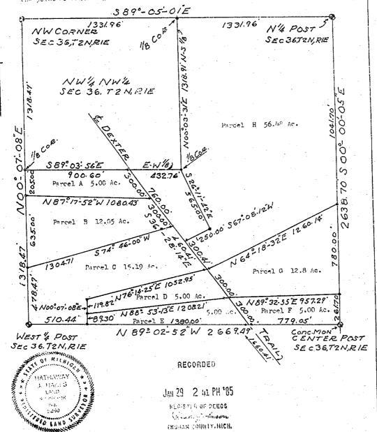
There by certify that I have surveyed the above property and that the ratio of closure of the unajusted field operation of such survey was 1/17000 and that this survey complies with Act 132 of P.A. of 1970.
