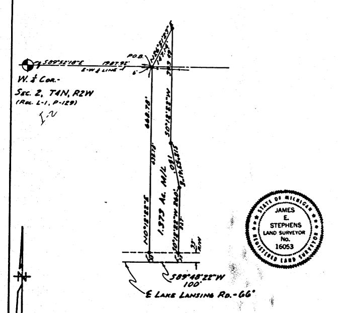
This survey complies with the requirements of Section 3, P.A. 132 of 1970, and that said survey was performed with an error of closure 1:5000
