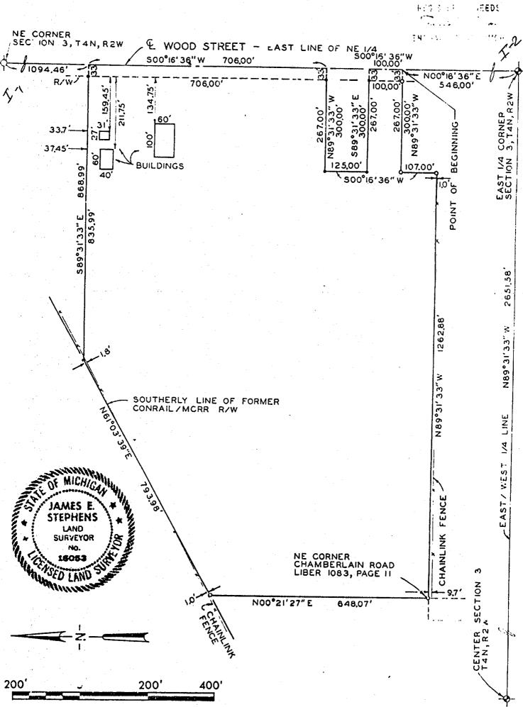
This survey complies with the requirements of Section 3, P.A. 132 of 1970. SCALE: 1"= 200" THE UNDERSIGNED LICENSED LAND SURVEYOR HEREBY CERTIFIES THAT A SURVEY WAS MADE UNDER HIS SUPERVISION OF THE PROPERTY SHOWN ON ANNEXED PLAT, AND THAT THE SKETCH INDICATES THE GMENSIONS AND ENCROACHMENTS OF SAID PROPERTY.
