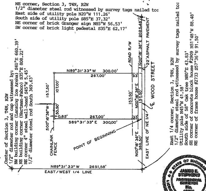
SCALE: 1"=100" This survey complies with the requirements of Section 3, P.A. 132 of 1970. THE UNDERSIGNED LICENSED LAND SURVEYOR HEREBY CERTIFIES THAT A SURVEY WAS MADE UNDER HIS SUPERVISION OF THE PROPERTY SHOWN ON ANNEXED PLAT, AND THAT THE SKETCH INDICATES THE DIMENSIONS AND ENCROACHMENTS OF SAID PROPERTY.
