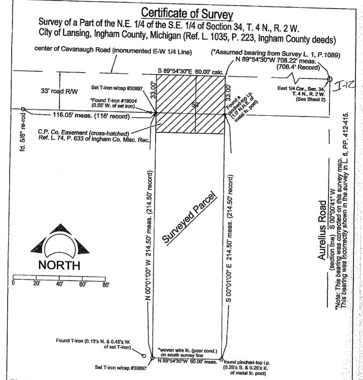
\*Note: The field work for this survey was done in 1989. The survey map field at that time (recorded in Liber 6, Pages 412-415 of Ingham County Certified Survey Maps) contained an error in the bearing shown on the east section line. This survey map is filed to correct that bearing.
