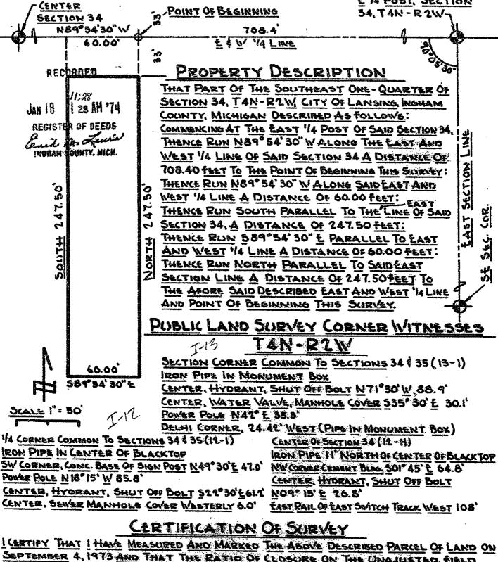
SEPTEMBER 4, 1973 AND THAT THE RATIO OF CLOSCIE ON THE UNAJUSTED FIELD OBSERVATIONS WAS NOT LESS THAN 1:5000 AND THAT ALL REQUIREMENTS OF P.A. 132 OF 1970 HAVE BEEN COMPLIED WITH.
