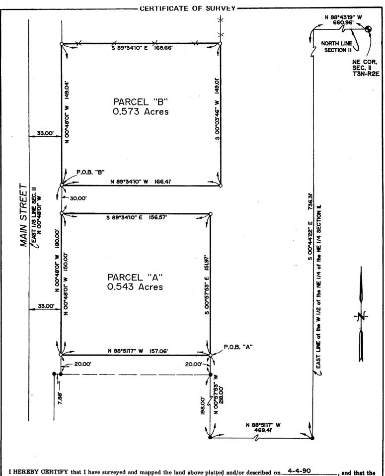
I HEREBY CERTIFY that I have surveyed and mapped the land above platted and/or described on 4-4-90, and that the ratio of closure on the unadjusted field observations of such survey was 1 N 73779, and that all of the requirements of P.A. 132 1970 have been complied with.
