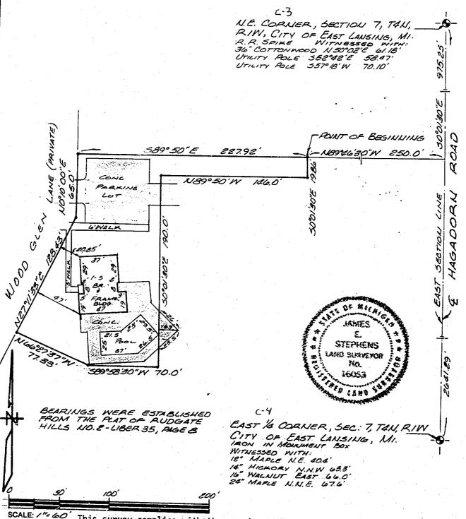
CALE: /"60 This survey complies with the requirements of Section 3, P.A. 132 of 1970 the undersigned registered land surveyor hereby certifies that a survey was made under his supervision of the property shown on annexed plat, and that the above sketch indicates the dimensions and encroachments of said property.
