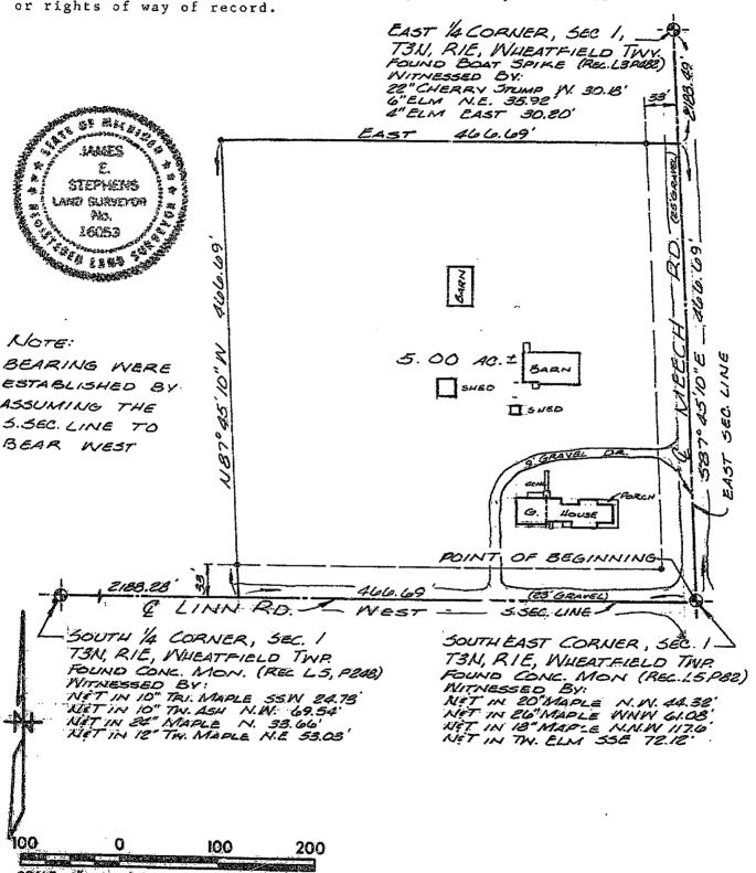
SCALE: /"=100 This survey complies with the requirements of Section 3, P.A. 132 of 1970 The undersigned registered Land Surveyor Hereby Centifies that a survey was made under his supervision of the Property Shown on annexed PLAT, and that the above sketch indicates the dimensions and enchoachments of said Property.
