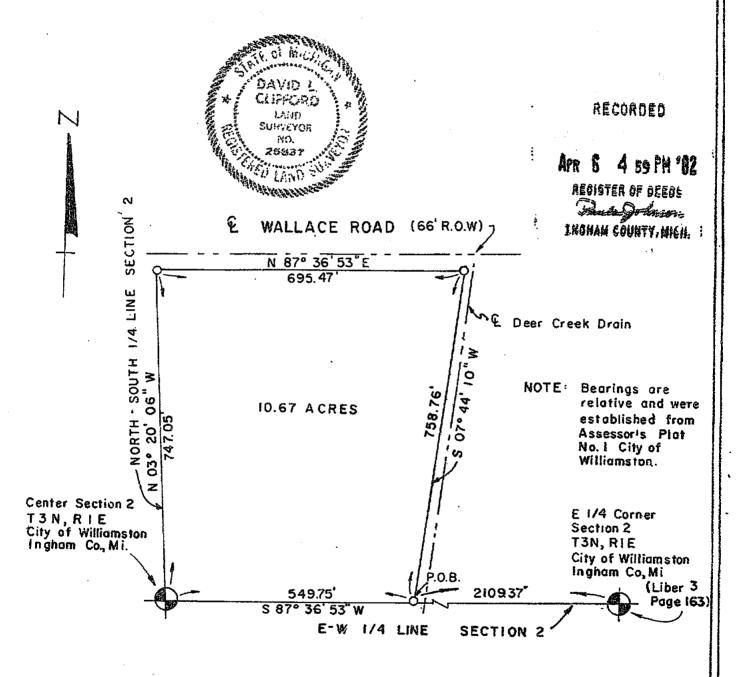
HEREBY CERTIFY THAT I HAVE SURVEYED AND MAPPED THE LAND ABOVE PLATTED AND OR DESCRIBED ON FEBRUARY 15, 1982, AND THAT THE RATIO OF CLOSURE ON THE UNADJUSTED FIELD OBSERVATIONS OF SUCH SURVEY WAS 1/16,520 , AND THAT ALL OF THE REQUIREMENTS OF P.A. 132 OF 1970 HAVE BEEN COMPLIED WITH.
