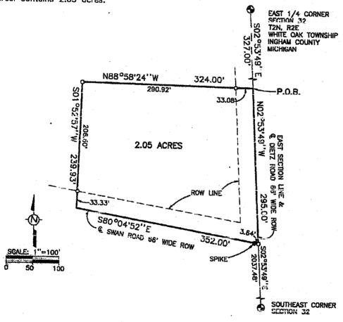
Bearings are based on the Michigan coordinate system of 1983, South zone. All dimensions are in feet.
