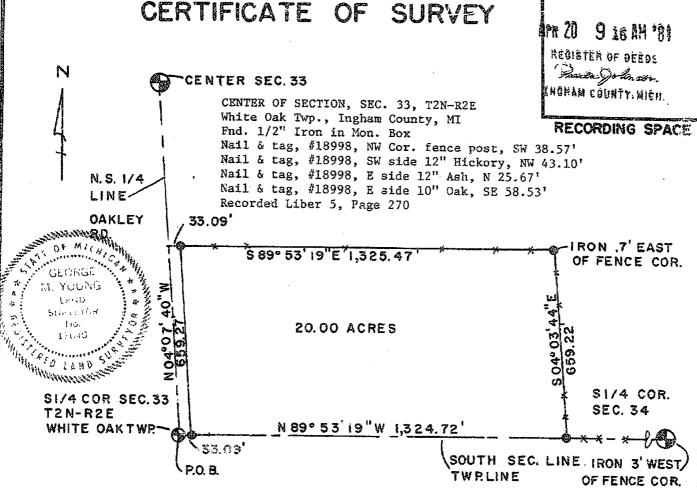
S 1/4 COR., SEC. 33, T2N-R2E White Oak Twp., Ingham County, MI Fnd. 1/2" Iron with cap Nail & tag, #18998, S side 18" Oak, W 33.41' Nail & tag, #18998, N side 18" Ash, ENE 24.57' Nail & tag, #18998, E side 16" Maple, NE 76.39' Nail & tag, #18998, W side 12" Ash, SE 44.50' Recorded Liber 5, Page 262
